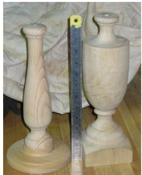
the stem to be attached. Check both sub assemblies for compatibility and pleasing design and correct before proceeding, if necessary. Drill holes in the base to allow for the cord to exit the stem and the side of the base as per the plan. Sand and polish or spray the base as for the stem and then thread the cord through the yet to be joined sub units. Ensure a sturdy fit between the stem and the base allowing 20 mm plus spigot length and fix with 5 minute epoxy or PVA glue.
