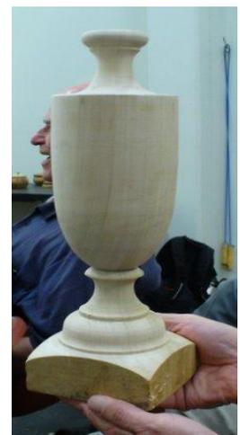
Choose wood for the lamp stem about 80 - 120 mm diameter and say 300 mm long and bore a hole 10 mm wide halfway through from each end. Try to centre these holes as deviation from the centre may mean that the cord will not easily pass the holes' join or
