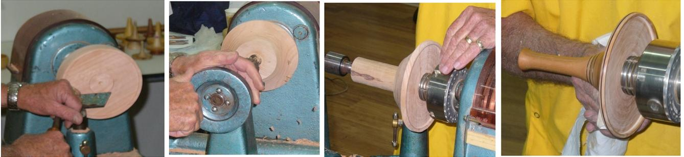
Remove the blank from the chuck and the chucking block. Reverse and chuck the blank in the recess made earlier. Reduce the thickness of the blank to 45 mm and drill a 25 mm diameter hole 15 mm deep to accept the handle's spigot. Check that this hole is 'square and clean'. Turn away some of the surplus wood on the back of the mirror block being careful not to encroach on the wood below the anticipated final curve profile.
