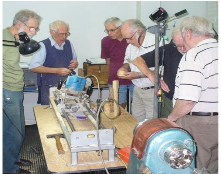
demonstrations of the machine producing spirals on various woods with interesting effect. The woods' finish is dependent upon the wood type and the cutter, with most spirals produced required relatively simple sanding for a standard finish.
