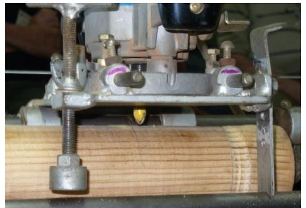
made around the blank, conversely if the blank remains stationary and the draw wire pulley only is turned a longitudinal cut will be obtained along the blank,
