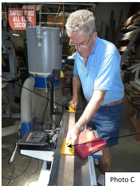
Downward pressure on board over out-feed table
