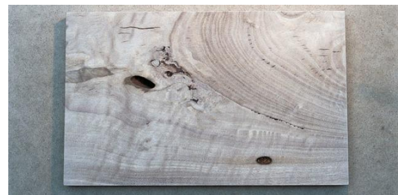
Larger defects may need to be cleaned up first.
