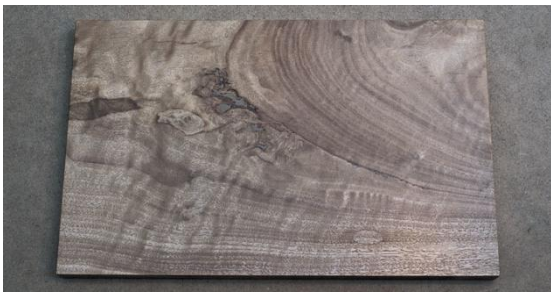
Fine cracks were filled with a sawdust and lacquer mixture.
