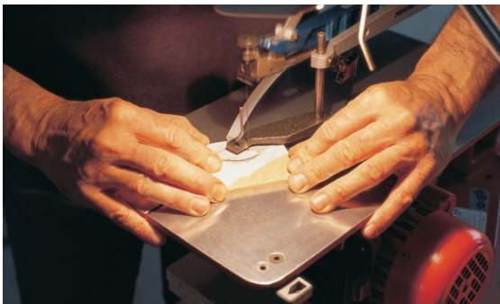
Cutting a plug on the scroll saw.
