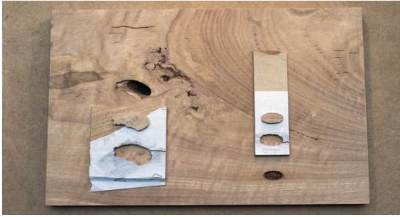
Match the grain and colour of the plug as closely as possible.
