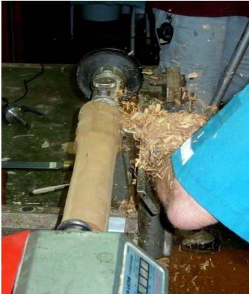
25 mm Ruffing Gouge. Although the eucalyptus wood is relatively much harder than the cypress there were no problems ruffing-down to a suitable finish at 40 mm diameter. Mark out at the critical lengths and using a sharp parting
