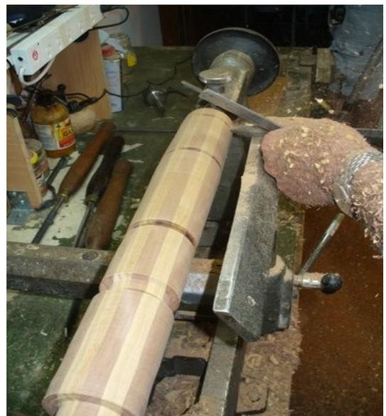
tool turn down a thin cut to the required diameter for its position along the chisel handle.
