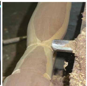
drilling of the the hole for the chisel tang at the tailstock end. Turn the spigot and the handle using a 12 mm detail gouge. Then progressing to the tailstock end turn to suit the copper 22 mm diameter by 20 mm ferule followed by turning the contour of the handle to the diameters set earlier with the parting tool. [Note the surplus length of billet between the the handle, and the spigot for the chuck jaws shown in the photos, will be discarded once the turning is complete].
