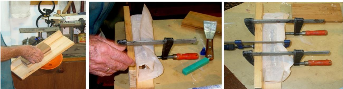
when clamped glue was extruded continuously from around all edges of the laminates. The glue used for the demonstration was exterior grade Aquadere white PVA.
