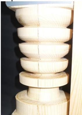
Remove the tape and using a flat chisel split the four lengths apart. Remove any surplus/loose paper, and reverse the four parts checking for fit etc and glue these together ensuring that the clamping retains the wood in the symmetrical/mirror positions for each face.
