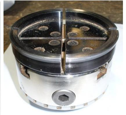
to 4 mm deep, and for these jaws dovetailed at 77 degrees. Take care to get the dovetail precisely formed, square and with all chips removed from the depth of the recess.
